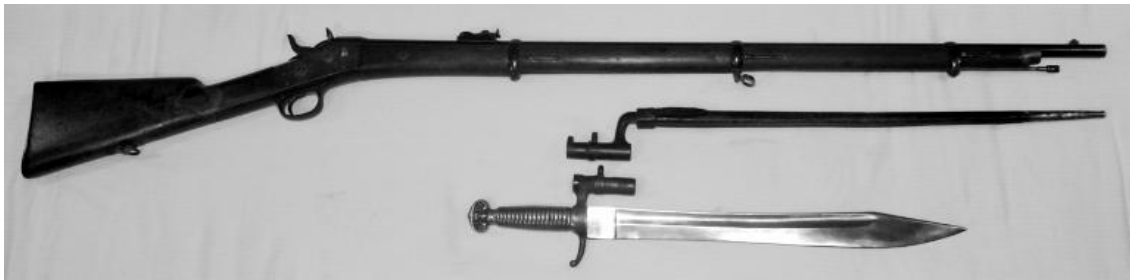
Variant M1858 bayonet and the Remington rifle to which it was adapted
