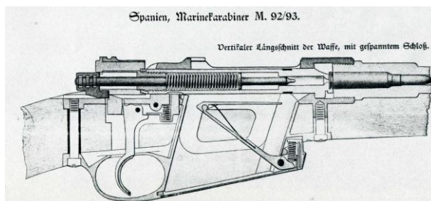
Factory diagram of the "Spanien, MarineKarabiner M.92/93"
