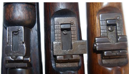
From left to right rear sights of M.91, M.93 and M.95 carbines.
