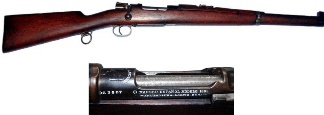
Model of 1893 Spanish carbine, 7 mm caliber, SN A3907, made by Loewe in 1894, and its markings.
