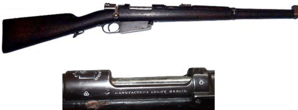
Model of 1891 "Modelo Español" carbine, 7.65 mm caliber, and its factory markings.
