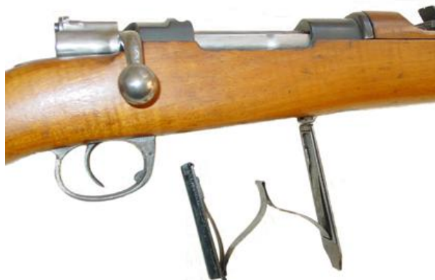
M.1916 Musketoon with magazine base plate opening latch.
