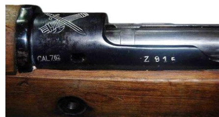
M.1916 musketoons converted to 7.62 NATO caliber in the 1950s, and for the Guardia Civil in the 1960s.
