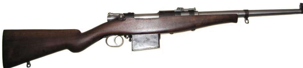
MANRESA carbine, SN 28, 7 mm caliber, with a 20 round magazine.
