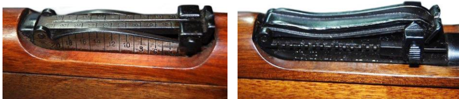
M.1916 Musketoon, 7mm caliber, with its M.1913 bayonet and the two types of rear sight, tangential to the left and Lange to the right.
