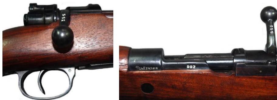
"Commercial" musketoons, SN 992, with curved bolt and no maker's markings.
