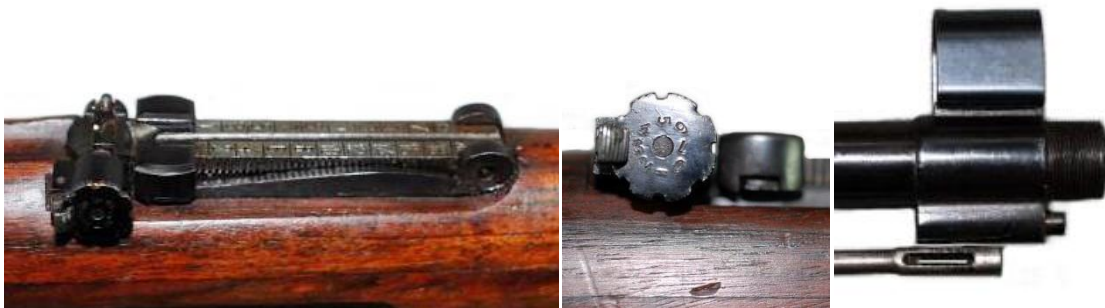
Experimental E.A-EXP.1 musketoon, its special rear sight, its threaded muzzle and, its markings.
