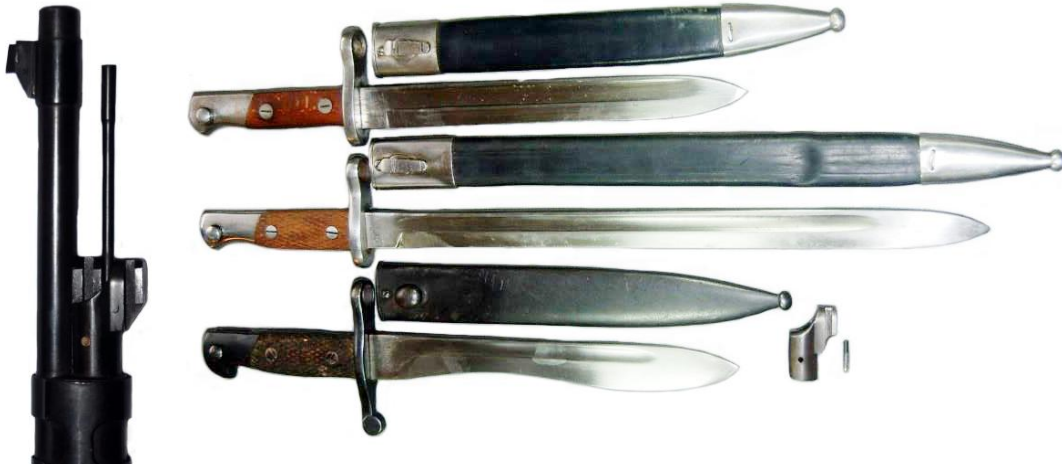
Detail of the M.1943's muzzle with adapter for the (from top to bottom) M.1893, M.1913, and M.1941 bayonets.
