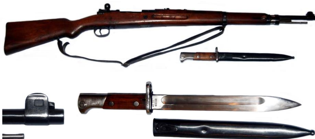
Air Force M.1944 musketoon, its emblem, its EA-prefixed serial number, and its M.1944 bayonet, made at the Toledo Factory.
