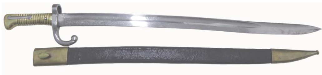
"Basque" made Chassepot sword-bayonet; 560 mm blade, 18 mm muzzle ring diameter, overall length 680 mm.
