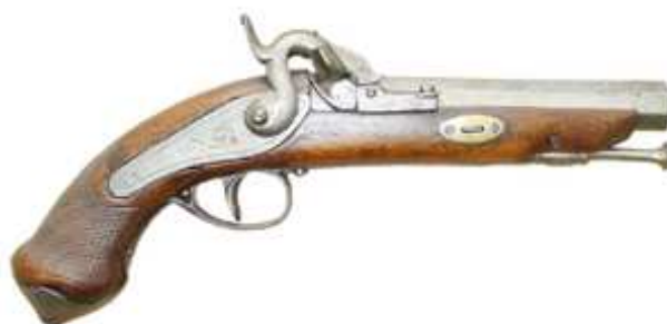
Commercial pistol with cast barrel 140 mm barrel, 17 mm bore diameter, with silver inscription: FABRICA / DE PEDRO ORBEA EN EIBAR / AÑO 1856 (Pedro Orbea, active from 1850-1870).
