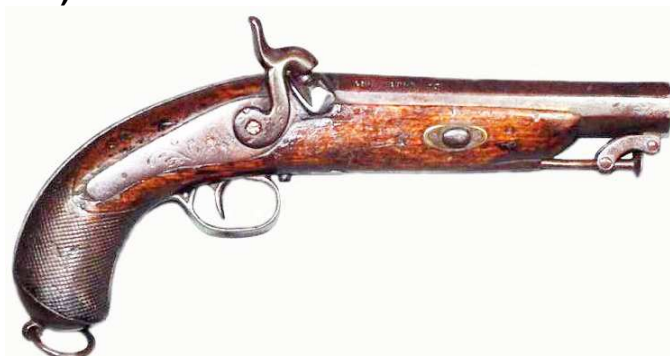
Percussion pistol of late manufacture; 150 mm barrel, full stock, 18 mm bore diameter, inscribed in silver: EN EIBAR / POR GASTELU / AÑO 1865 (Gregorio Gaztelu, 1860-1870); It bears a number 98, issue number to armed personnel, on its stock, probably constables (Photo H. J. Meruelo)
