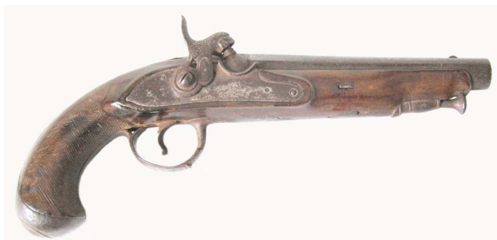
Commercial Eibar pistol, circa 1830; 170 mm barrel, 17 mm bore diameter, inscribed “ De Herraduras ” in silver, referring to the type of forging used in its manufacture.
