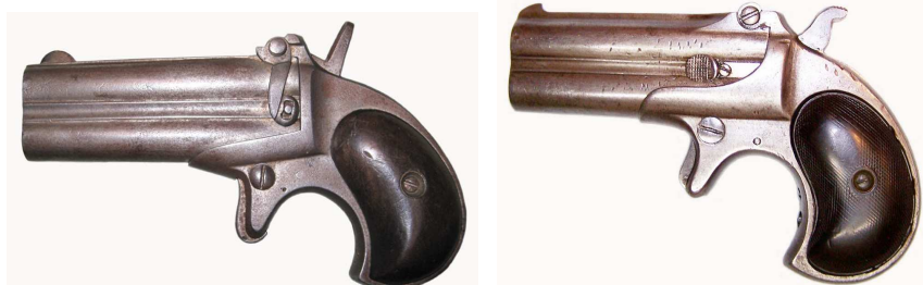
Unmarked Eibar copy of the Remington Double Deringer with automatic extractor on the left, and, on the right, marked “REMINGTON ARMS. U.M.C. ILION NY”, n° 442, with manual extractor.
