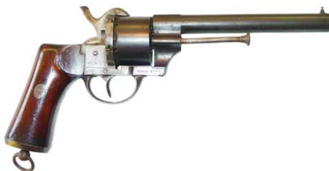
Mod. 1863 Lefauchaux revolver, 6 shots, 12 mm caliber, barrel length 155 mm, marked "OVIEDO", dated 1868 and with SN 3849
