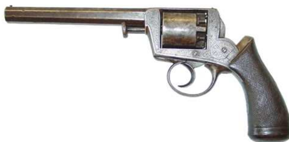
1851 Adams revolver, 5 shots, 9.5 mm caliber, barrel length 160 mm, with silver inscription "POR MANUEL GARATE EN EIBAR", and serial number 36.
