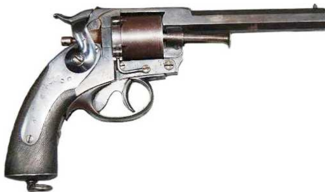
Model 1864 Navy Kerr revolver, transformed to metallic cartridge use, as the Model 1870 (Photo H. J. Meruelo)
