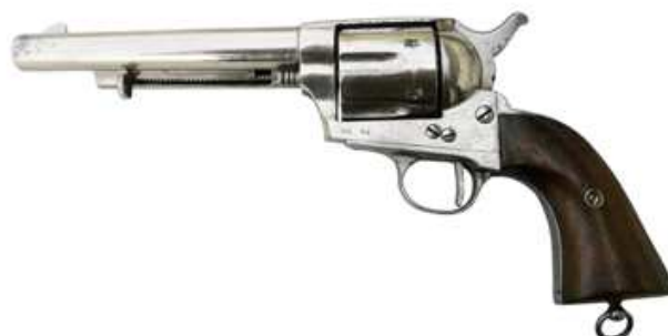
Single action, six shot, 44 caliber, Eibar “Colt 1873” revolver; Barrel length 150 mm, marked “SYSTEM REVOLVER V. ARIZM. MANUFACTURER OF FIREARMS” (Vicente Arizmendi, 1880-1894)
