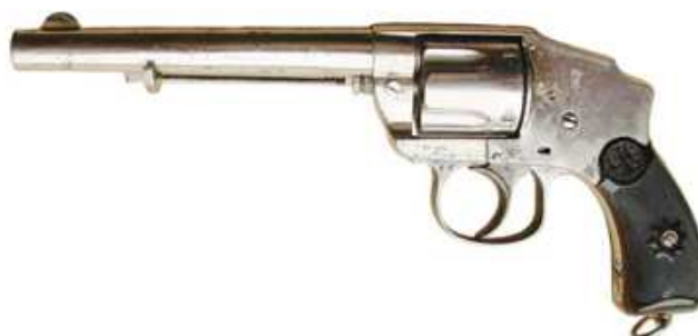
Five shot, 38 caliber, “Hammerless” revolver; Barrel length 134 mm, marked “COLT’S PT. F. A. MFG. C° / HARTFORD CT. U.S.A”, serial number 53845; Logo “LGC” on grips (Larrañaga, Garate y C a )
