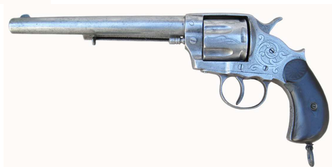
Six shot, 44 caliber, double action, Eibar “Colt 1878”; Barrel length 191 mm, marked “COLT’S CARTRIDGES ARE THOSE THAT” / “FIT BEST THE EUSKARO REVOLVER”, serial number 21, unknown maker.
