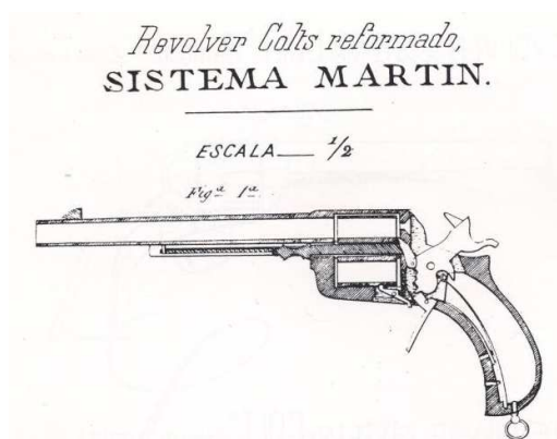
Drawing of the “Colts reformado sistema Martin” with folding trigger, patented in 1887 by Martin Antonio Bascaran.
