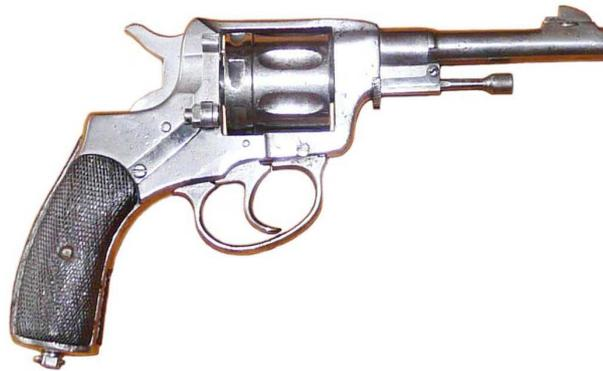
Eibar “Nagant” revolver, without cylinder advance system; Seven shot, 7.62 mm Nagant caliber; Barrel length 104 mm with “F. Arizmendi y Goenaga”’s logo; Offered in their 1912-13 catalogue as the “Officer’s Model”.
