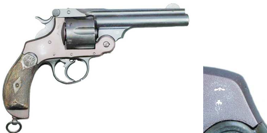
Revolver model “Pistol O.P with five inch barrel, No 1 Mark 1” marked: “MANUFACTURA ESPECIAL DE REVOLVERES / GARATE ANITUA Y C a . EIBAR (ESPAÑA)”, with “GAC” logo, and with the British Army’s “broad arrow” acceptance marking (Photo H. J. Meruelo)
