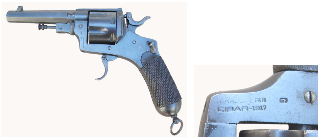
Six shot, double action, 10.35 mm caliber, Md.1889 Bodeo revolver, marked: “S. AROSTEGUI / EIBAR 1917”
