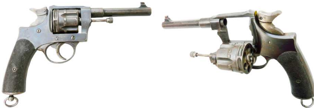
Six shot, double action, “Modèle 1915”, 8 mm Lebel caliber revolver, with “AE” logo on the frame (Antonio Errasti).
