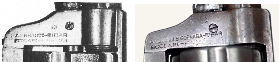
Antonio Errasti and “Arizmendi & Goenaga” trade marks on Md. 1889 Bodeo revolvers, both also marked “SCOLARI – ROMA 1916”.
