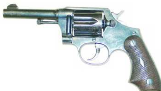
“ATCSA” revolver, 38 caliber, six shot, 4” barrel, serial number 85, marked “ATCSA / PAT. 130396 / MADE IN SPAIN”
