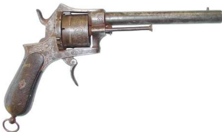
Single piece frame, double action, 6 shot, 12mm caliber pinfire Lefauchaux revolver; Barrel length 169 mm; inscribed in silver: "CAÑON DE ACERO / F a DE UNCETA Y BARRENECHEA / EIBAR", serial number 24.
