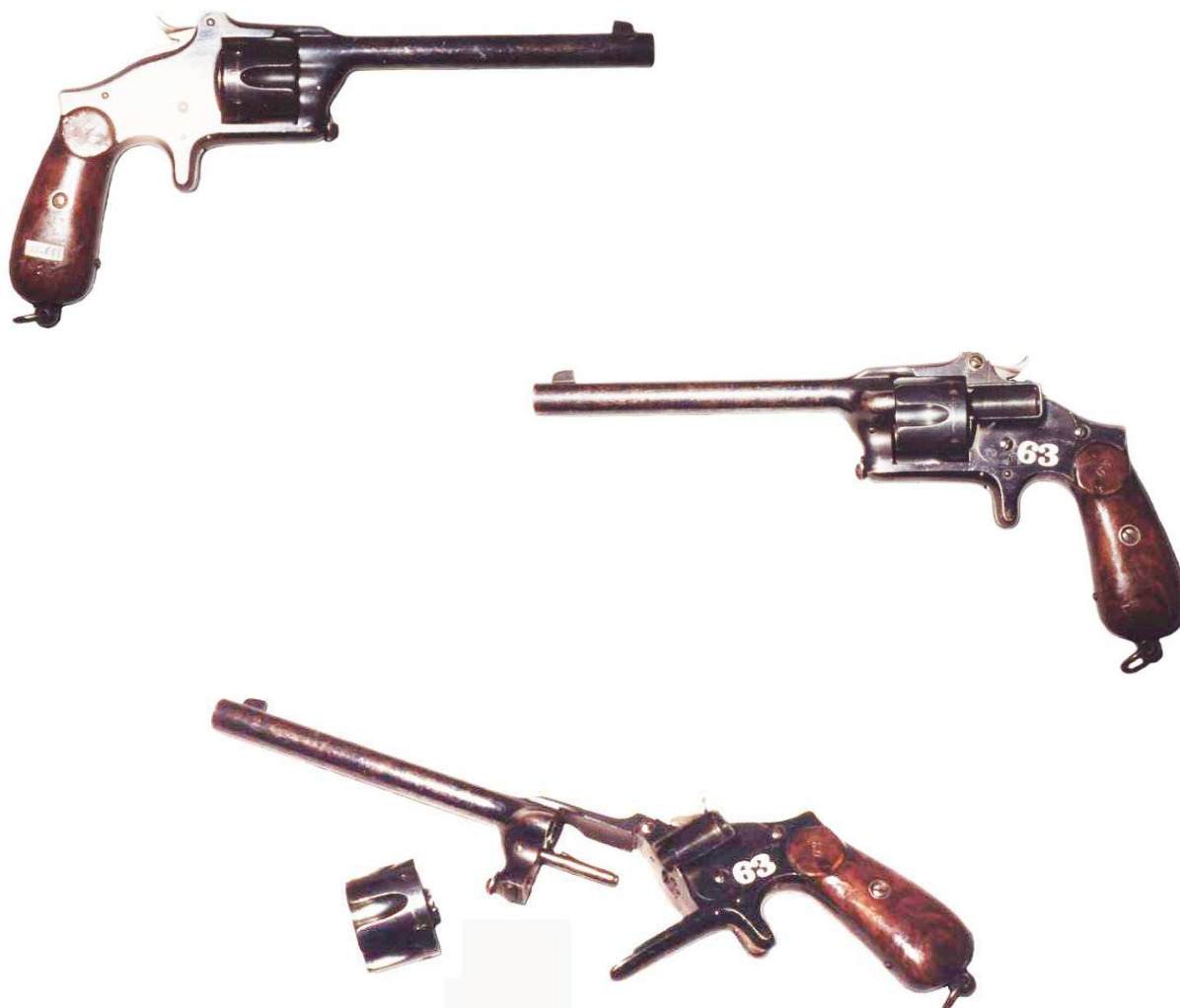
First project Piñal revolver with the Ibarra gas extraction system; Six chambers, barrel length 162 mm; Item number 5815 of the Army Museum Collection.
