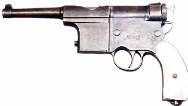
7 mm "Charola y Anitua" pistol with a six round stripper clip fed magazine
