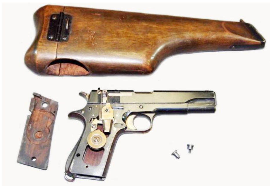
Model MD STAR pistol with fire selector, rate reducing mechanism, and wood holster/shoulder stock (Photo P. Bello)
