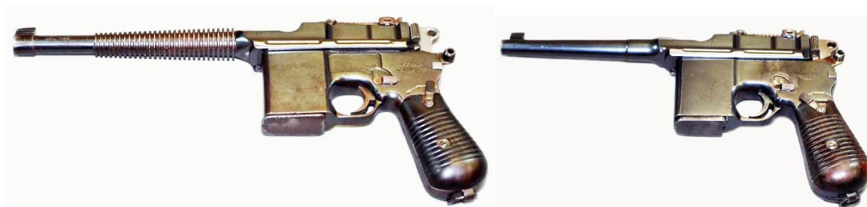
MM 34 pistols, as offered by the firm of “Beistegui Hermanos” in their two variants, with and without, barrel cooling fins (Photo P. Bello)
