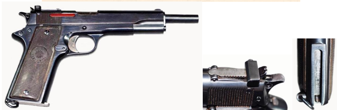
Model A STAR “pistol-carbine” advertisement, and 7.63 mm caliber Model A STAR “pistol-carbine”, SN A5949, with adjustable tangent sights and slot for attachment of a wooden holster/shoulder stock (Photo H. J. Meruelo)
