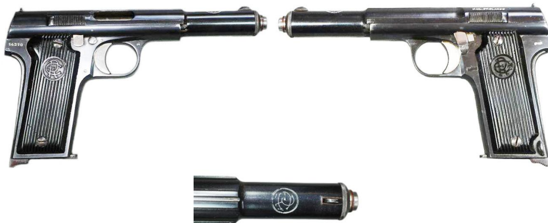
Model 1921 9 mm RE (República Española) pistol made in Alginet, Valencia; Around 15,000 were made; Marked “CAL 9m/m Largo”, logo “RE”; (Photos H. J. Meruelo)
