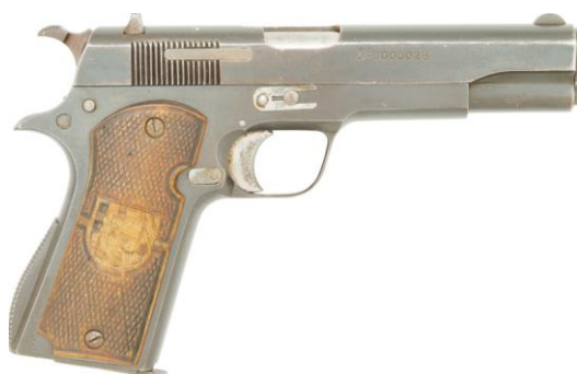
ISARD pistol, SN 28, variant of the "1 st Model" lacking the grip safety. (Photo Leonardo M. Antaris)
