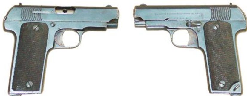
“RUBY” pistol, cal 7.65 mm, 9 shot, 88 mm barrel, marked: GABILONDOS Y URRESTI, EIBAR-RUBY CAL. 7,65
