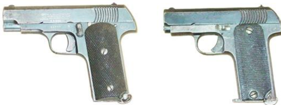
Nine shot, “Ruby-type” pistols; Left marked: S.A. ALKARTASUNA / FABRICA DE ARMAS / GUERNICA, logo “ALKAR”; Right marked: 7,65 1914 MODEL AUTOMATIC PISTOL / M.ZULAICA & C° EIBAR
