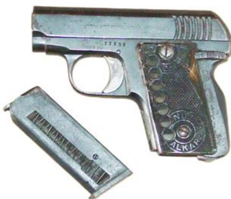
Seven shot, 6,35mm cal, “Eibar-type” pistol with grip safety and see-through holes to allow seeing the number of rounds left in the magazine; Specimen with ALKAR trademark and: AUTOMATIC PISTOL MODEL NEW ALKAR and CAL. 6,35 and NEW ALKAR on the grip panels; It was also marketed under the trademark MANUFACTURA DE ARMAS DE FUEGO- GUERNICA, which succeeded the ALKAR S.A after its destruction in a fire.
