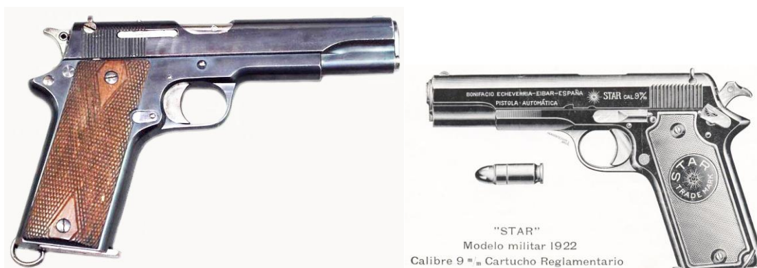
Left: STAR M 1922 9 mm Largo pistol, SN 24862, marked: BONIFACIO ECHEVERRIA – EIBAR (ESPAÑA) followed by the bursting STAR logo and “STAR” CAL 9 m/m 38; preceded by the Guardia Civil emblem on the frame and on the matching number magazine; Right: STAR M1922 advertisement. Notice that only the thumb safety remains, the grip safety having been eliminated. (Photo H. J. Meruelo)
