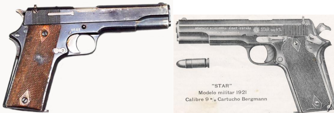
Left: STAR M 1921 9 mm Largo pistol, SN 5625, marked: BONIFACIO ECHEVERRIA – EIBAR ESPAÑA followed by the bursting STAR logo and “STAR” CAL 9 m/m 38; and preceded by the Guardia Civil emblem on the left frame and on the matching number magazine; Right: STAR M1921 advertisement. Notice the thumb and grip safeties similar to the M1911 Colt. (Photos H. J. Meruelo)
