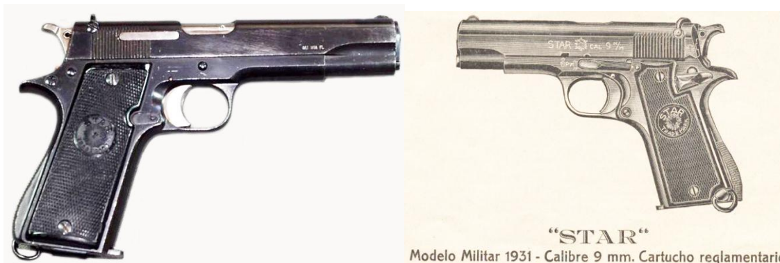
Left: STAR M1931 9 mm Largo pistol, SN 166806, marked: Bursting STAR logo followed by STAR AUTOMATIC PISTOL CAL 9 m/m 38; and BONIFACIO ECHEVERRIA – EIBAR – ESPAÑA. This specimen is a commercial Model A; Right: STAR M1922 advertisement. Notice similarity to the Colt M 1911 A1. (Photo H. J. Meruelo)
