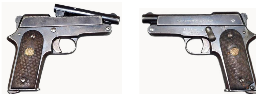
Seven shot, 7,65 mm caliber, Sharp-Shooter pistol, SN 11225, marked: SHARP-SHOOTER PATENT No 68027 with logo “OV” in the grips (“Ojanguren y Vidosa”, dealers and distributors) and early Eibar rampant lion proof. (Photo H. J. Meruelo)
