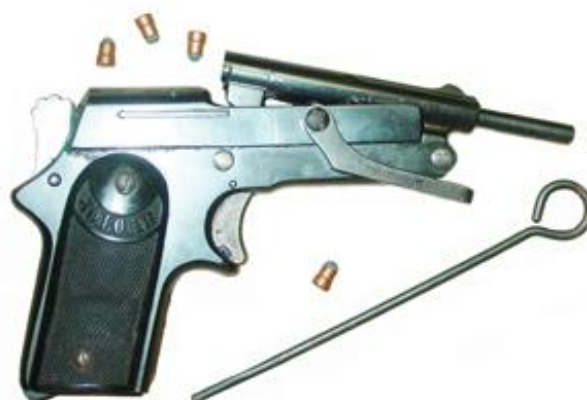
Cal 6.35 mm JO.LO.AR pistol with caliber reducing barrel insert in position; It used the 4mm M20 rounds made by the “Rheinisch-Westfalische Sprengstoff A.G”
