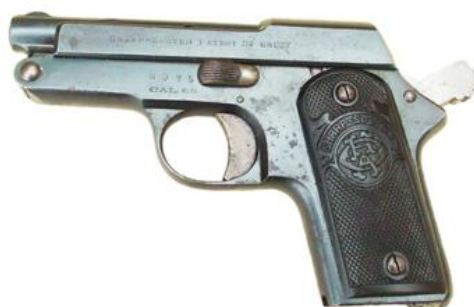
SHARP SHOOTER pistol, cal. 6.35 mm , cocked and locked; Markings: SHARP-SOOTER PATENT 68027 / CAL 6,35, logo SHARP SOOTER HCA (Hijos de C. Arrizabalaga); Swiveling the safety lever back releases the barrel which then tips up and a round can be inserted
