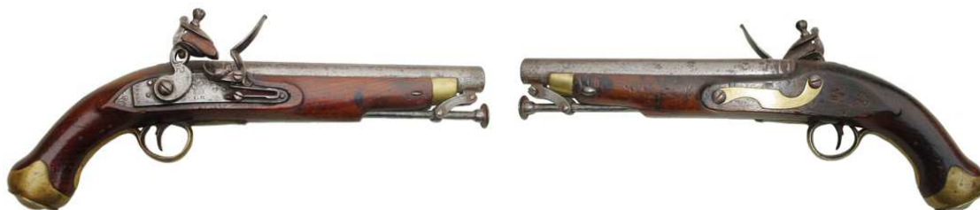
English “New Land Pattern” cavalry pistol; 16 mm. (“de a 23”) caliber, 225 mm. long barrel.
