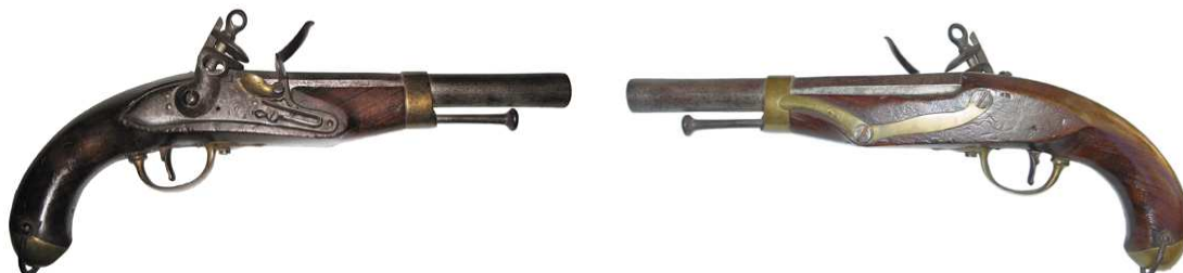
Spanish cavalry pistol, model of 1815; 18 mm. (“de a 17”) caliber, 230 mm. long barrel.
