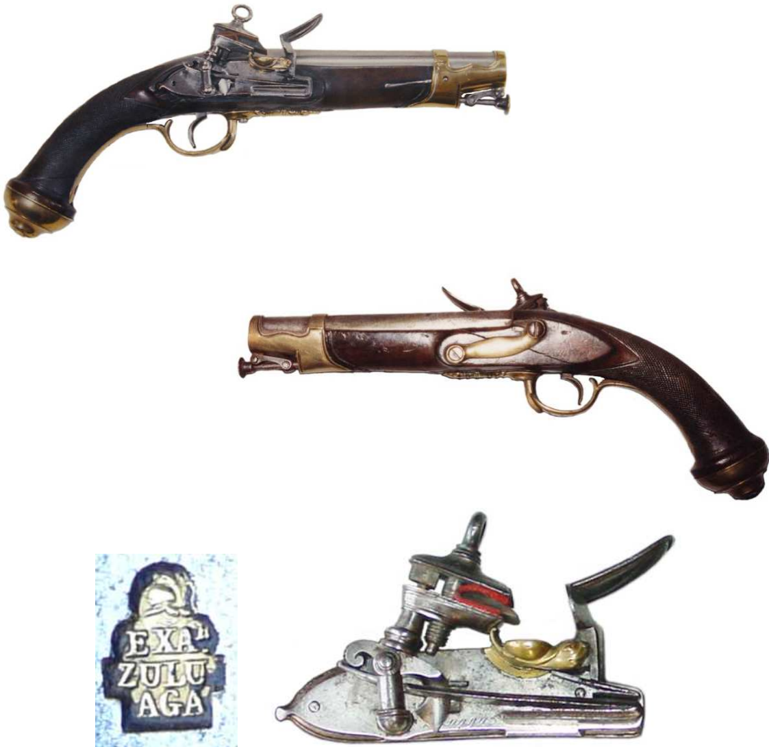
Cavalry Pistol of the model used by the Major Officers of the Royal Corp of “Guardias de la Persona del Rey”; 178 mm long, 18 mm (“de a 17”) caliber barrel, marked under helmet “EXAR/ZULU/AGA” (Examinador Ramon de Zuloaga, Placencia), bearing the Royal Arms and the inscription “ RI. Cuerpo de Guards. de la Persona del Rey ”; Spanish lock, inscribed “Zuluaga” and the triggerguard inscribed “Ramon Zuluaga”.
