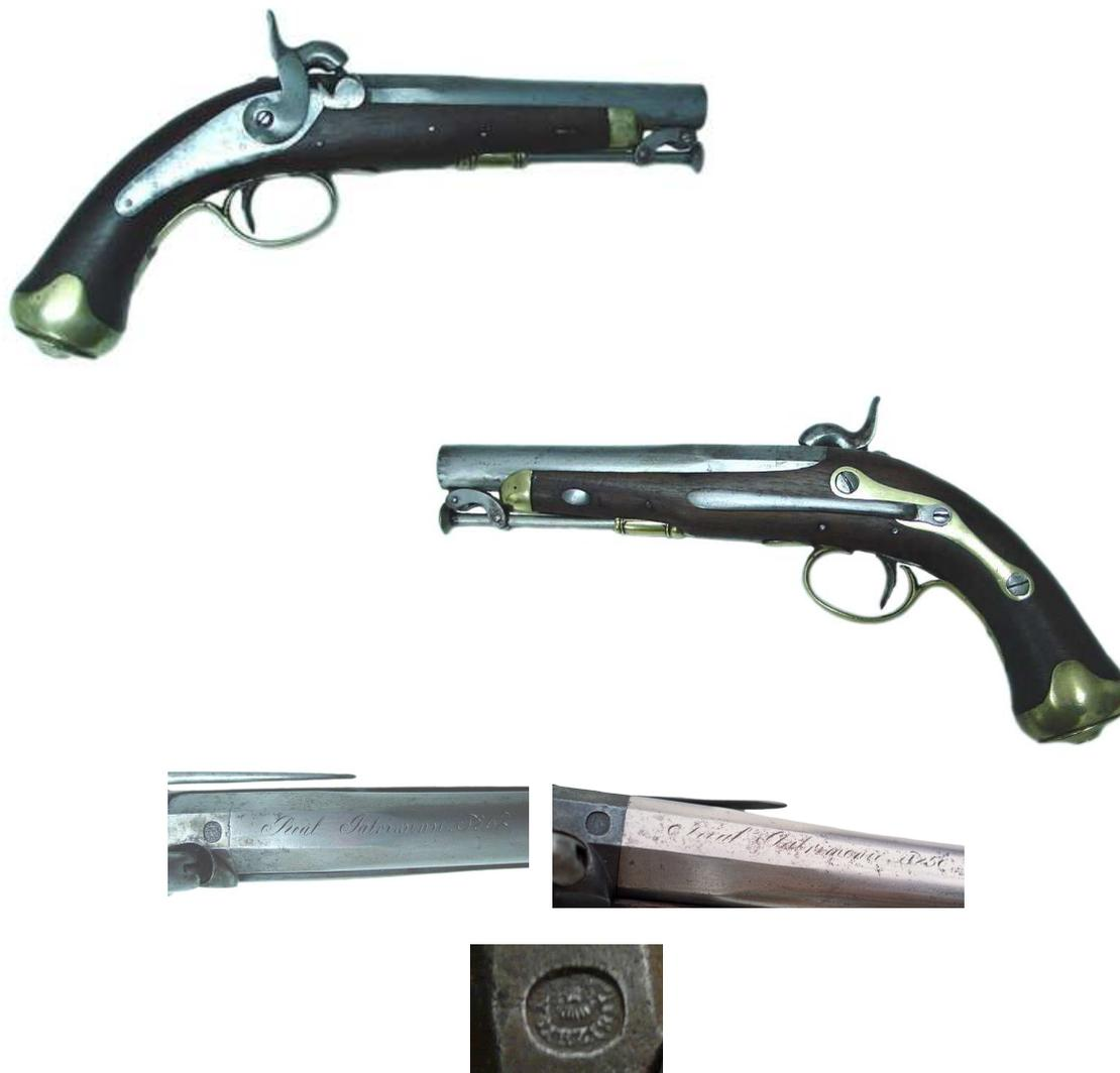
Police model pistol; 169 mm long, 16.5 mm caliber (“de a 21”) barrel; Marked “YBARZABAL” in an oval surrounding a starburst, inscribed “*Real Patrimonio 1862*”; Percussion lock with inverted swivel mechanism lacking any markings; Articulated ramrod holder, full stock with brass fittings and an iron belt hook; Overall length 320 mm; In a similar specimen the barrel is inscribed “*Real Patrimonio 1850*”; E. Gorostiza collection.
