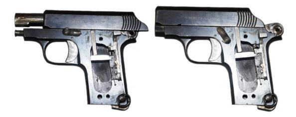
Left: The slide hold-open device, engaged; Right: The safety, below the hammer, in the downward "safe" position.
