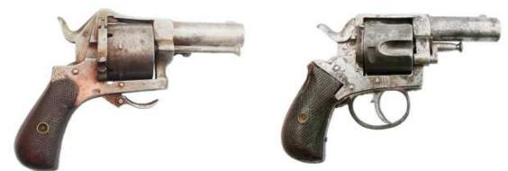
Double action "Bulldog" five shot revolver. LEFT: for 12 mm caliber pin fire cartridges; Barrel length 63 mm; Marked: "BULL-DOG", unknown maker. RIGHT: for .44 caliber center fire cartridges; Barrel length 63 mm; Marked: "BRITISH / BULLDOG", unknown maker.
