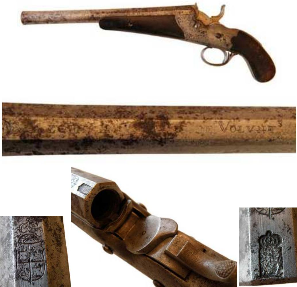
**Pistol with Remington rolling block system, built using a Spanish bore-type barrel, for 16 gauge shells, with a 29.21 cm long barrel, 18.74 mm caliber, with illegible gunsmith's marking, engraved with the Royal Arms and the inscription "REGIMto. DE CABALLA. DE VOLUNTs".**
