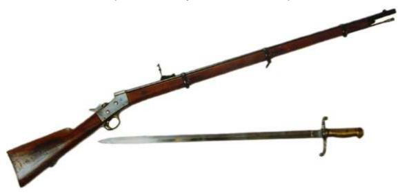
Model of Remington rifle and sword-bayonet which equipped the Infantry Company of the Corp of "Guardias de S.M. el Rey", Amadeo I; Specimen dated 1870, manufactured at the Oviedo Factory; 900 mm long barrel, caliber 11 mm, bearing a sword- bayonet attachment lug; The bayonet blade is double edged on two tables and is inscribed "Fca. DE TOLEDO / AÑO DE 1871"; Specimen number 4759 of the Collection of the Museo del Ejército.
